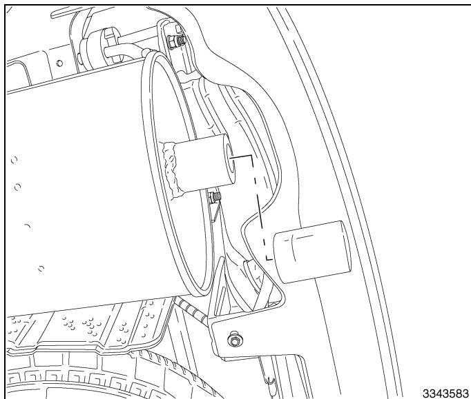
5. Slide the chrome exhaust tip onto the muffler tip with the pilot hole down.
